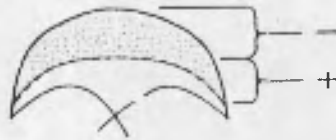
Excursion of a Flattened Diaphragm
